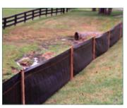
designated to filter out sediment from construction site run-off, yet allow clean water to pass through. Tenax Silt Fence is pre-assembled with hardwood stakes securely attached at 10-foot intervals and packaged in 100 lineal foot rolls.
